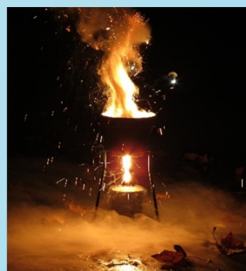
The thermite reaction gives off so much heat that the iron formed is molten
